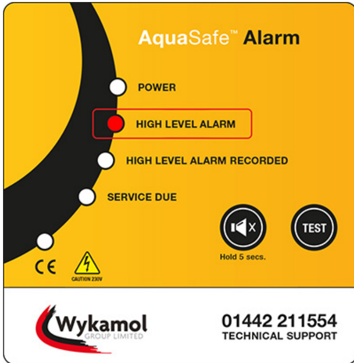
Fig.12 The high level alarm indicator
