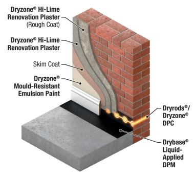
Thinner thicknesses may be used (e.g. when matching in with existing plasterwork) but maximum moisture salt resistance is achieved when the total plaster thickness is at least 25 mm (2 layers).
